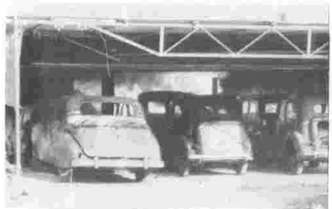
Fig. 17. Car park fire test
