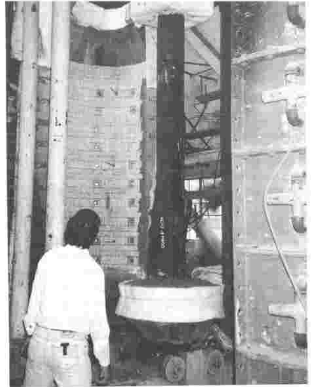
Fig 5 Thor Column prior to fire testing at LPC
