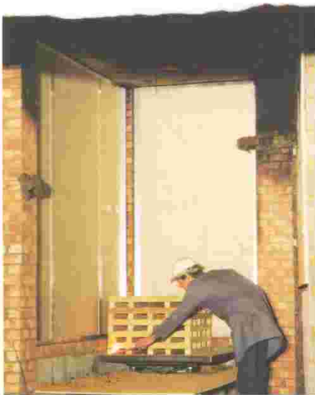
Figure 1 Corner-wall test rig showing panels and crib before test
