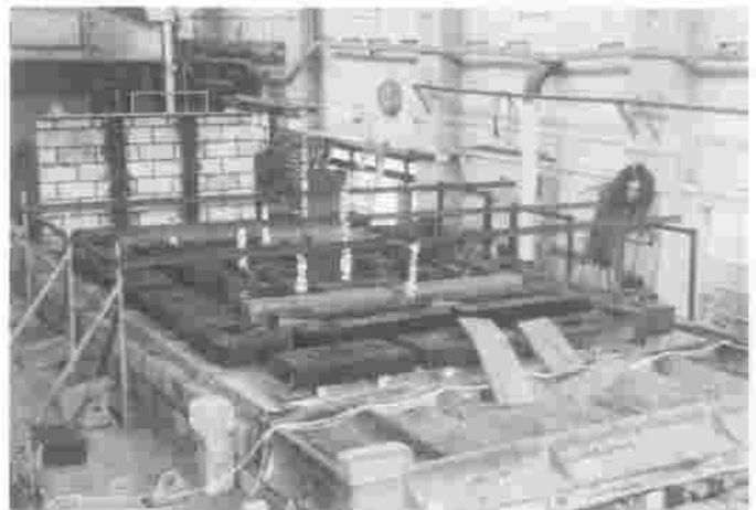
Fig 4. Loading on composite deck in a fire test
