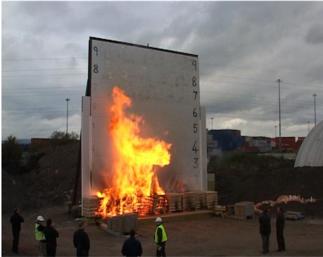
Tall flames near start of test
