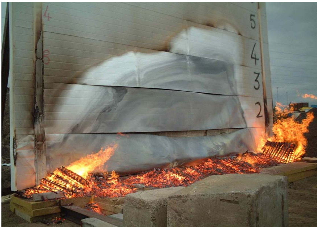
Delamination of fire-exposed panel faces due to thermal bowing, fire dying away.
