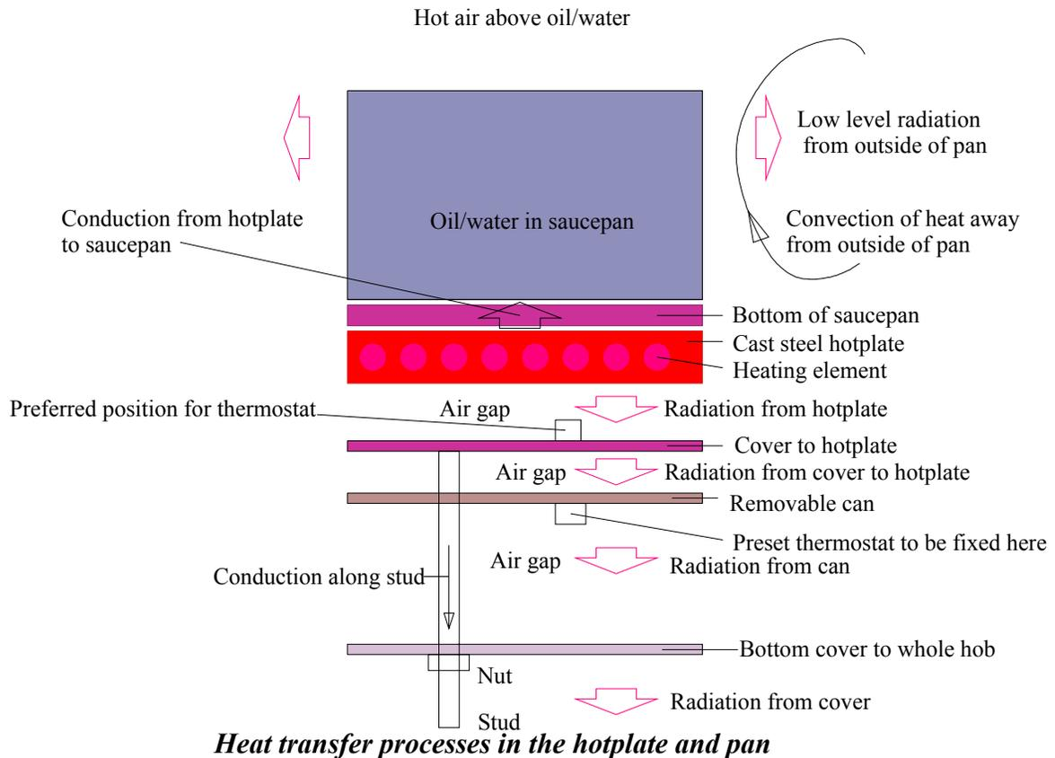
Furthermore the choice of operating temperature of the thermostats could not be tuned too finely as there was a lag between the heating of the heating element embedded in the cast steel hotplate and the heating of the oil. The heat transfer processes were complicated, as shown in the diagram, and of course the diagram does not indicate time-based phenomena such as phase lag. The proving tests were done on a spare hob both in the test laboratory and in the hostel
