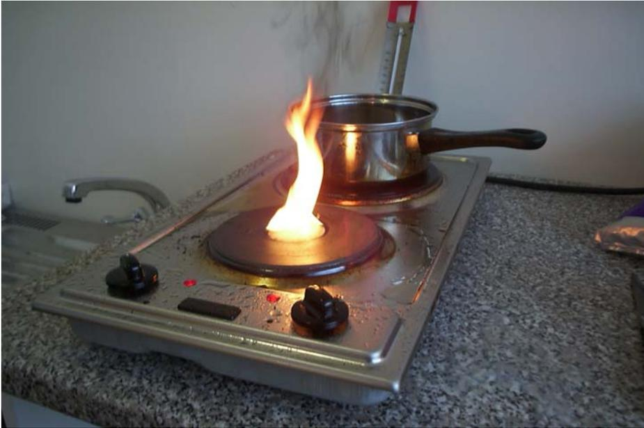
*Test on unmodified hob with both hotplates at maximum power after small amount of oil was poured onto centre of hotplate. A major spillage could produce a chip-pan fire*
