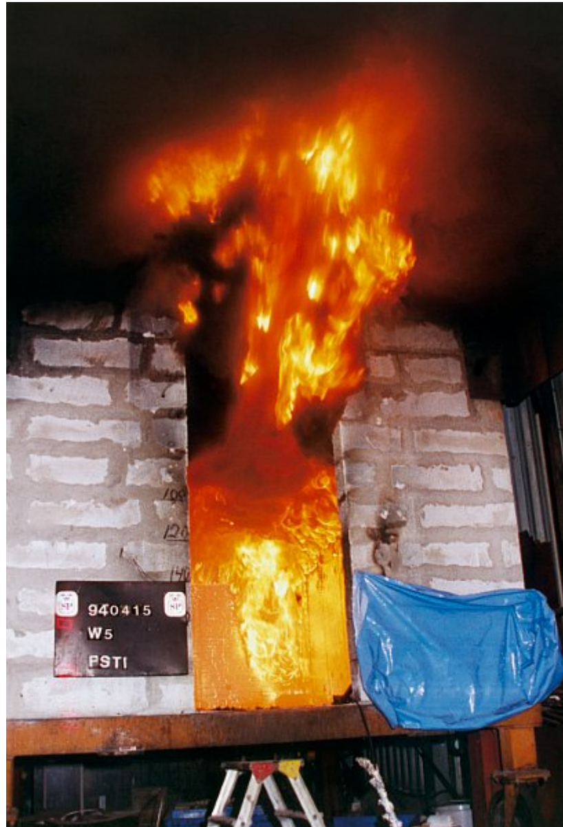
Typical example of flashover in the ISO 9705 reference room test (flames emerge from doorway, upper surfaces of specimen involved in fire)
